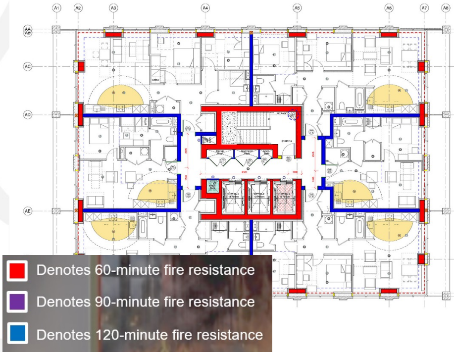
Example fire strategy drawing showing compartmentation layout
